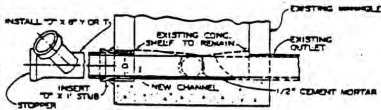
SECTIONAL ELEVATION B-B CHANNEL BASE
